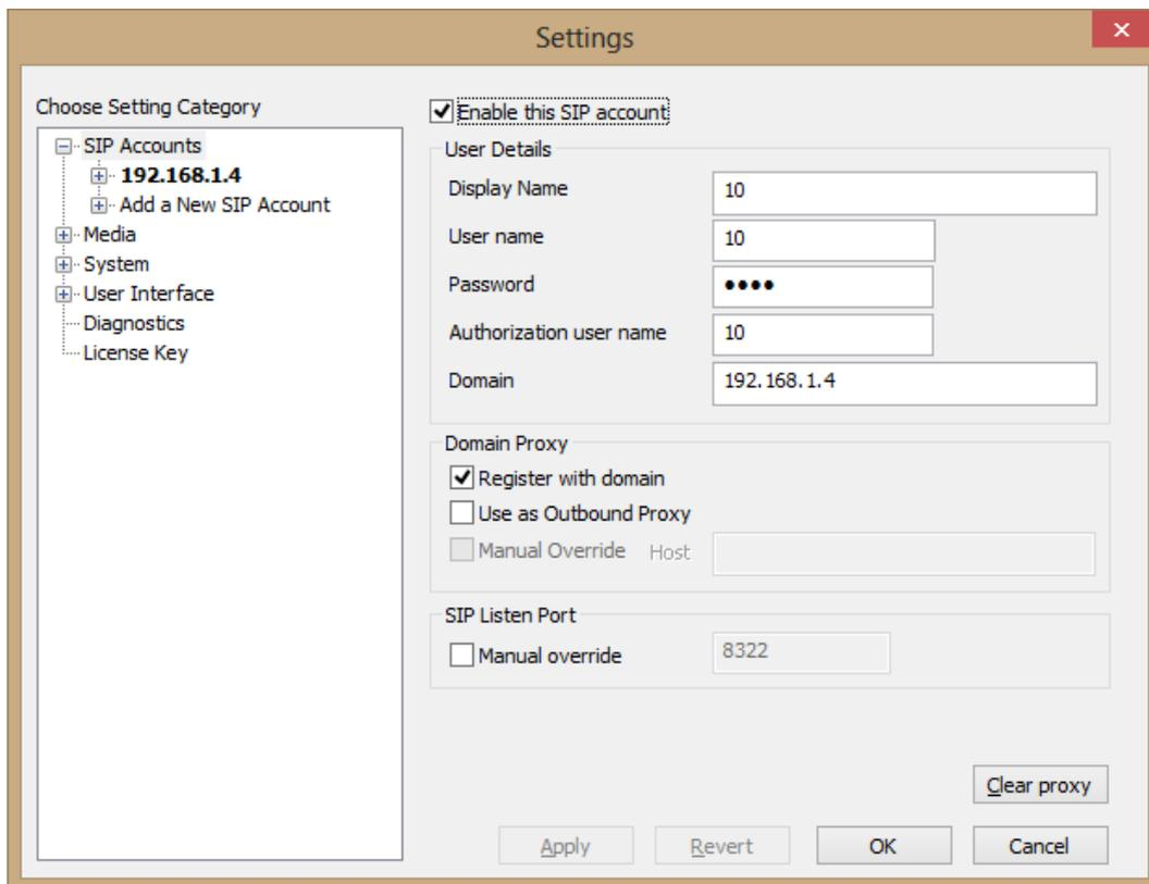
**Figure - 11.** eyeBeam Configuration
